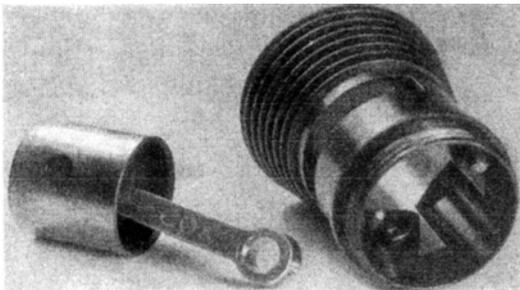
alloy conrod. At the same time the cylinder bore was increased by .006 in. to take full advantage of the 2.5 cc displacement limit and rotary-valve timing was altered to give earlier opening.
