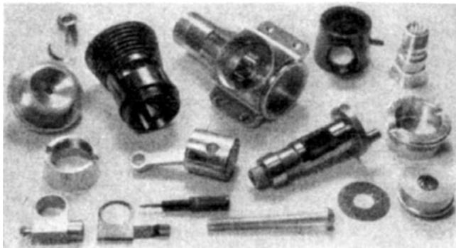
Close-up illustrates new single exhaust port and three large transfer flutes in place of the usual symmetrical arrangement of dual opposed exhaust ports and dual opposed transfer flutes. These effectively reduce exhaust port area by just over 30 per cent from the Mk. I Special .15.
