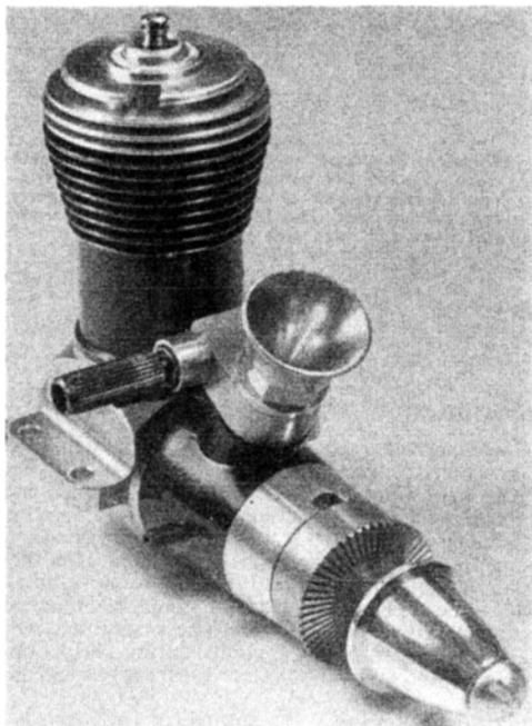
**I**N view of the new FAI rule extending the obligatory use of standard methanol/castor fuel to the FAI free-flight power class, we shall, in future, be making a point of using standard fuel when testing engines in this category. Accordingly, our report this month on the Mk. II version of the Cox Special .15, includes performance curves obtained from tests using straight 3 to 1 methanol and castor oil fuel.
