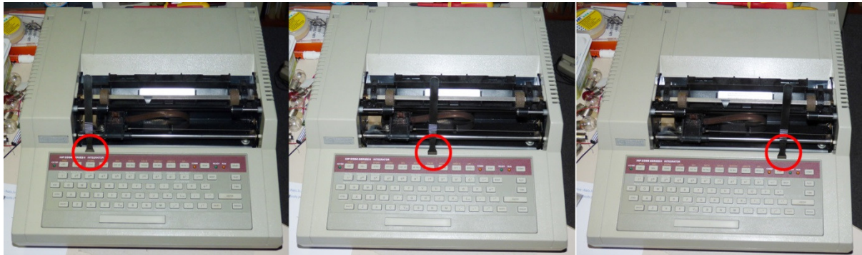
Figure 1: Three latches are located at the upper edge of the keyboard plate. Push down with a proper pry tool of about 20-40 mm width to unlock them.
