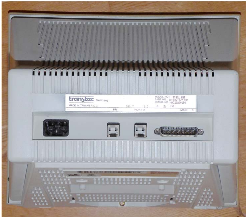
Figure 7: The rear view of the main unit (swiveling foot removed) shows the printer port and a second serial port as well as the DB-25 connector for the first serial port.
