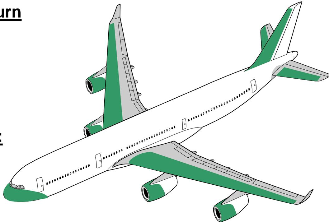
**10% net drag reduction** is targeted for application of laminar flow technology
