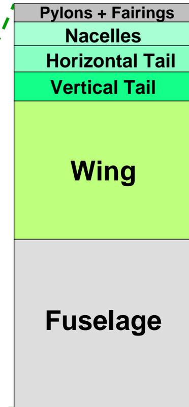
> **Wing** offers (besides fuselage) highest potential for friction drag reduction
