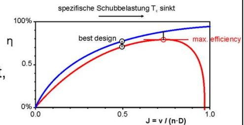
The graph shows the maximum possible efficiency (blue) according to momentum theory and the efficiency of a real propeller versus advance ratio (roughly == flight speed).
