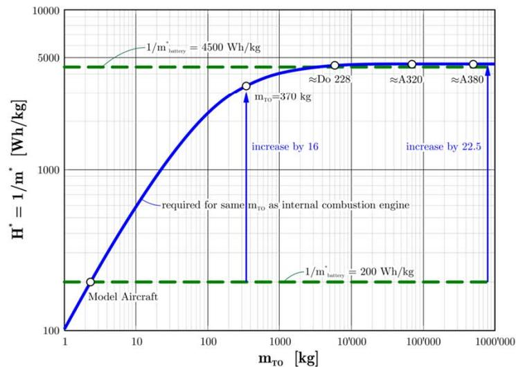
We ask for exactly the same performance (flight time or range) of battery electric powered and kerosene powered aircraft.
