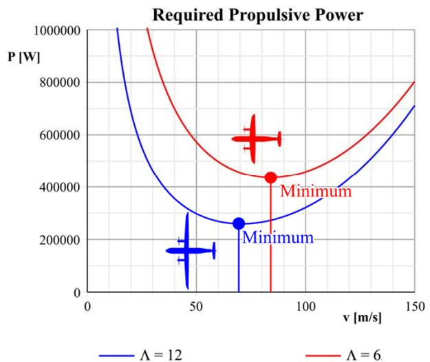
Any aircraft has propulsive power requirements. These depend on aircraft shape, mass and flight speed.
