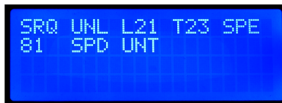
Figure 2: The output on the LCD shows the SRQ event sent by a HP 3478A digital voltmeter. The serial poll result 81 has bits 0 („Single Trigger“), 4 („Front/Rear“ switch in „Front“ position) and 6 („External Trigger“) set.
